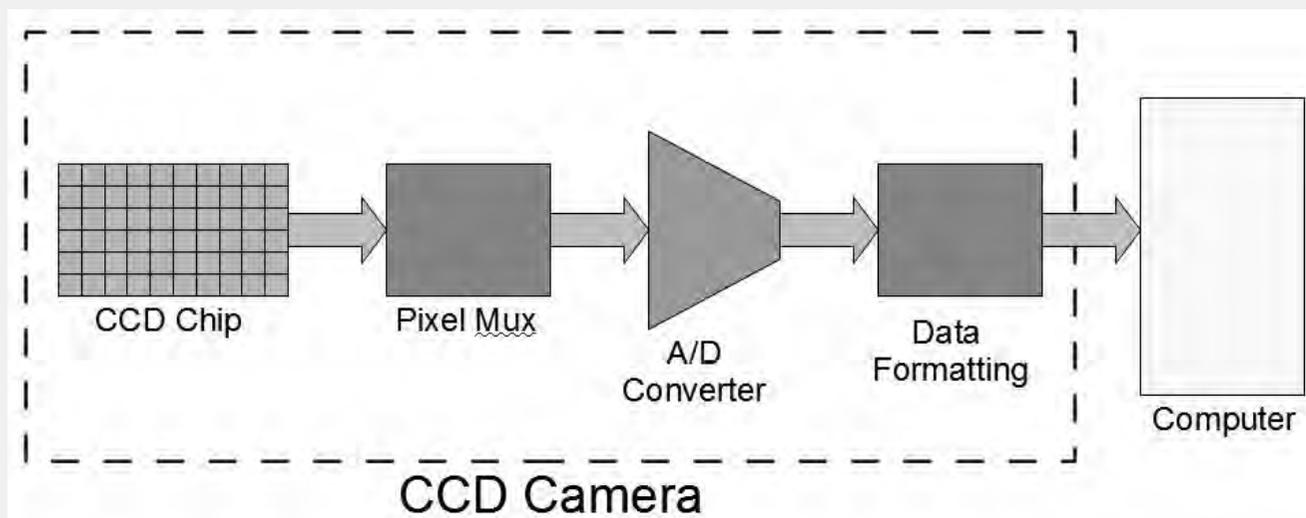
Components of a CCD Camera
