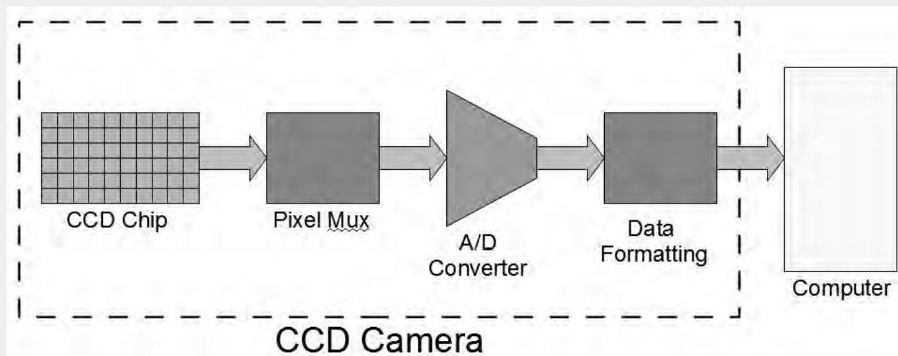
Components of a CCD Camera
