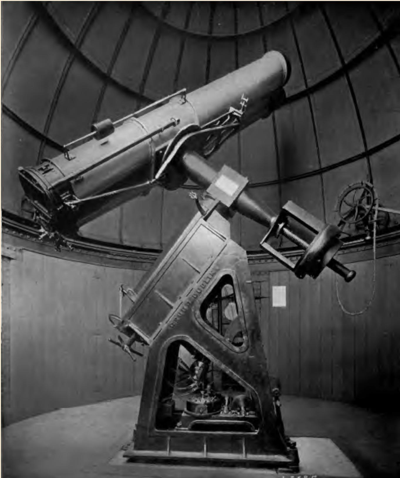
**Greenwich Observatory Astrograph, built by Sir Howard Grubb, c1891**
