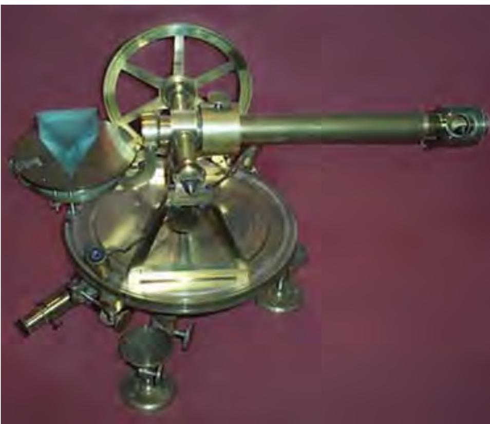
In 1814 Joseph Von Fraunhofer (1787-1826) rediscovered 'Wollaston's Forgotten Lines', using an instrument known as a Spectroscope (left). This essentially simple device consisted of a prism on a rotating table, with a microscope through which the spectrum of the light source can be seen. By rotating the prism different parts of the spectrum can be seen. A scale of wavelengths is marked on the table, which can be read with the aid of a simple micrometer.
